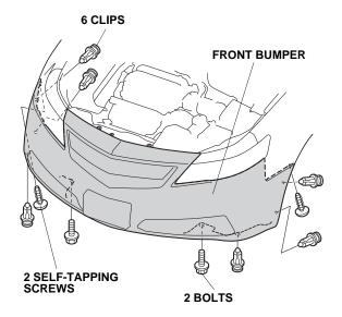
7. On each side, release the 11 hooks, and gently pull the front bumper out from the body.
