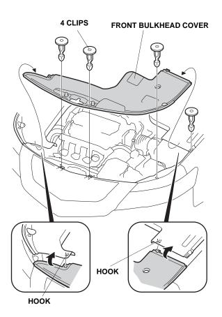
2. Remove the four clips, and raise the engine compartment right cover.
